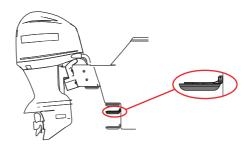
The transducer can be mounted on a transom bracket. With this mounting option the transducer can be in the water when you are on plane, or can be mounted so it is only in the water when you are moving at trolling speed.
