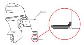
The transducer can be mounted on a transom bracket. With this mounting option the transducer can be in the water when you are on plane, or can be mounted so it is only in the water when you are moving at trolling speed.
