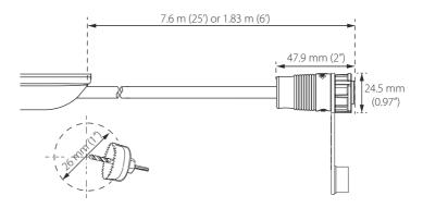
A 26 mm (1") diameter hole is recommended for cable connector clearance.
